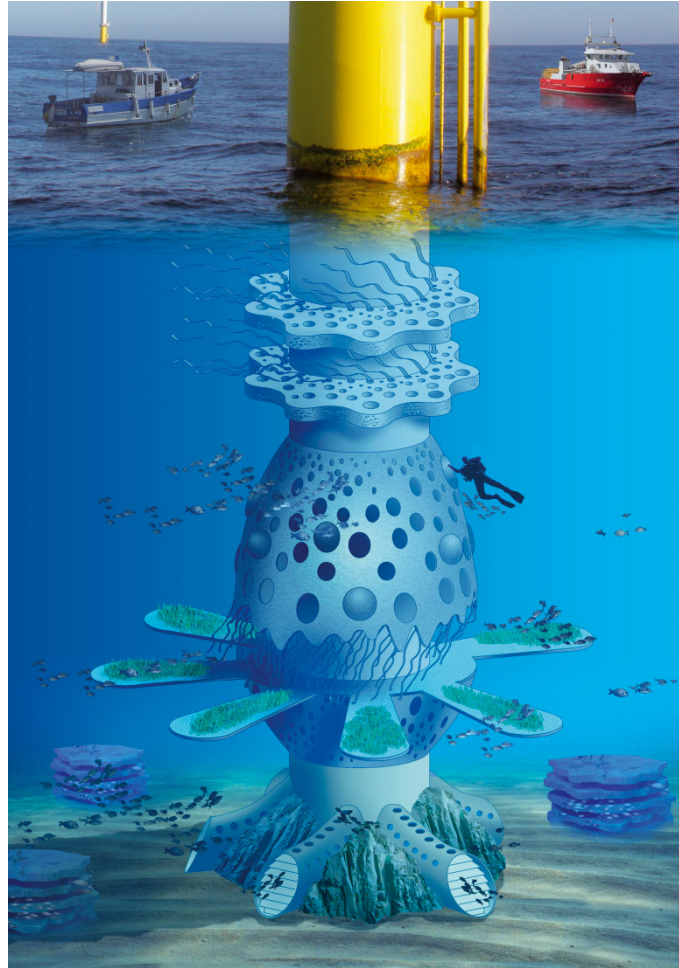
Fig. 1. Eco-designed offshore foundation for fishes, sea-grass and multi-use purposes: diving, fishing, tourism, etc. © Egis Eau/ Sylvain Pioch and Jean-Luc Féron.
