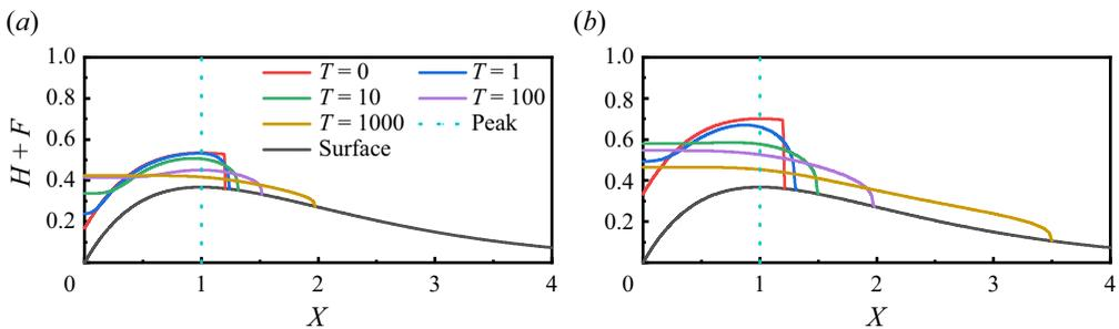
Figure 6. Temporal evolution of a viscous fluid over a two-dimensional linear-exponential surface under different release volumes and initial lengths. Panels show (a)  $M = 0.2$ ,  $X_0 = 1.2$ ; (b)  $M = 0.4$ ,  $X_0 = 1.2$ .
