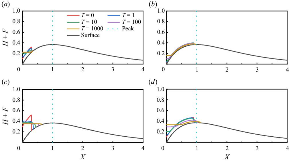
Figure 2. Temporal evolution of a viscous fluid over a two-dimensional linear–exponential surface under different release volumes and initial lengths. Panels show (a)  $M = 0.03$ ,  $X_0 = 0.3$ ; (b)  $M = 0.03$ ,  $X_0 = 0.9$ ; (c)  $M = 0.09$ ,  $X_0 = 0.3$ ; (d)  $M = 0.09$ ,  $X_0 = 0.9$ .
