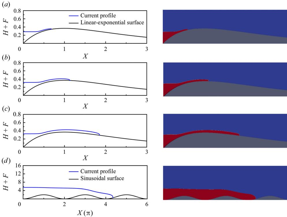
Figure 12. Qualitative comparison between the numerical solutions of low-dimensional models and CFD results for two-dimensional propagation over linear-exponential and sinusoidal surfaces ( $t = 1 \text{ s}$ ).
