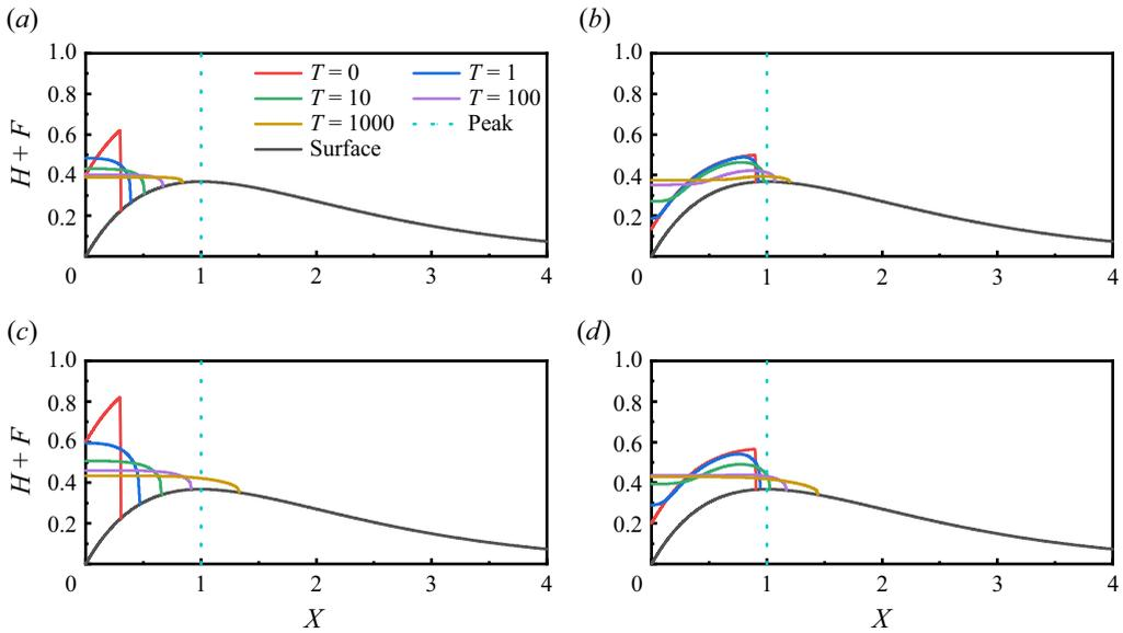
Figure 4. Temporal evolution of a viscous fluid over a two-dimensional linear-exponential surface under different release volumes and initial lengths. Panels show (a)  $M = 0.12$ ,  $X_0 = 0.3$ ; (b)  $M = 0.12$ ,  $X_0 = 0.9$ ; (c)  $M = 0.18$ ,  $X_0 = 0.3$ ; (d)  $M = 0.18$ ,  $X_0 = 0.9$ .
