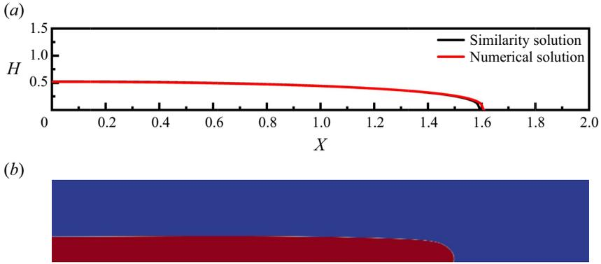
Figure 17. Comparison of current profile for axisymmetric propagation over a horizontal straight surface ( $t = 1$  s). (a) Similarity and numerical solutions; (b) CFD results.
