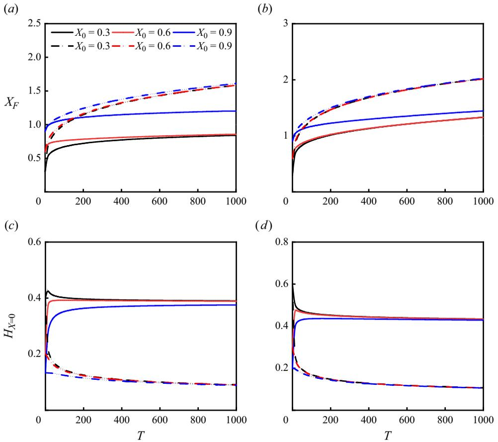
Figure 5. Comparison of the current front and height at the origin between a horizontal straight surface and a two-dimensional linear-exponential surface under different release volumes and initial lengths. Panels show (a,c)  $M = 0.12$ ; (b,d)  $M = 0.18$ ; solid line, linear-exponential surface; dashed line, horizontal straight surface.
