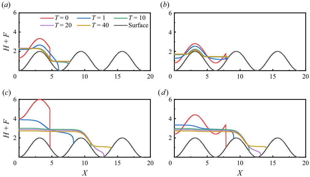
Figure 9. Temporal evolution of a viscous fluid over a two-dimensional sinusoidal surface under different release volumes and initial lengths. Panels show (a)  $M = 2\pi$ ,  $X_0 = 1.5\pi$ ; (b)  $M = 2\pi$ ,  $X_0 = 2.5\pi$ ; (c)  $M = 6\pi$ ,  $X_0 = 1.5\pi$ ; (d)  $M = 6\pi$ ,  $X_0 = 2.5\pi$ .
