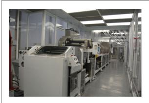
Solarmer's roll-to-roll pilot production line for the manufacture of organic photovoltaic modules.
