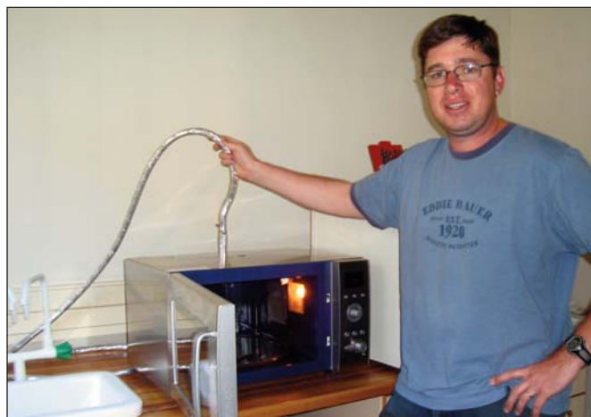
Thompson holds a gas purge line used to cool an installed infrared sensor after modification of a microwave furnace at the University of Western Cape.
