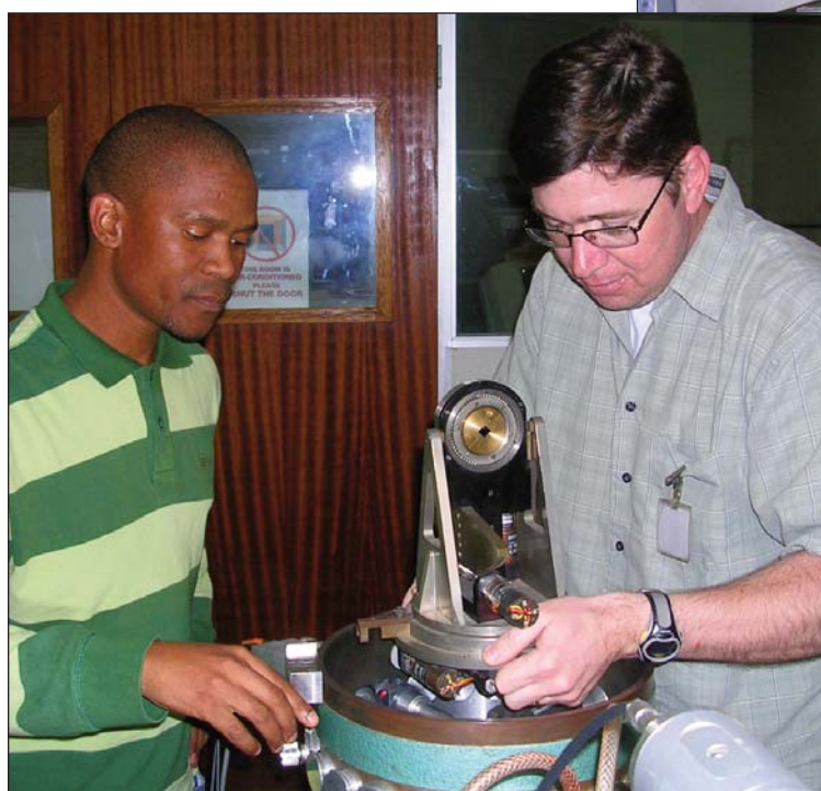
An iThemba Labs ion beam analyst Phillip Sechogela (left) and Thompson insert a sample mounted to a three-axis goniometer into an RBS analysis chamber.
