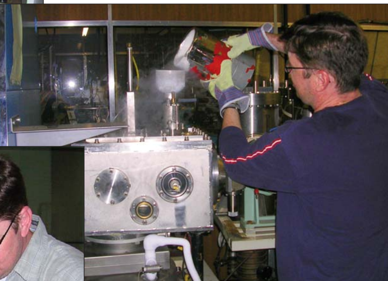
Thompson fills a liquid nitrogen reservoir on the Varion/Extrion ion implanter at iThemba Labs (Gauteng). Liquid nitrogen is used to cool samples during implant
