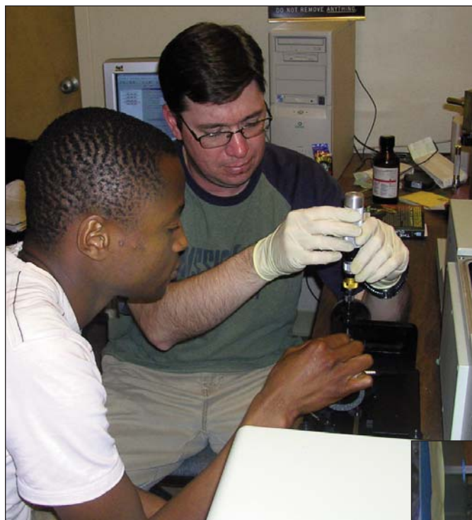
Thompson and Tile clamp a sample to a germanium crystal prior to performing mid-infrared–Fourier transform infrared spectroscopy.
