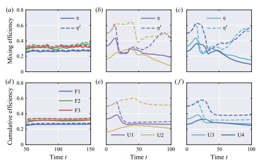
Figure 9. Time series of (a-c) instantaneous and (d-f) cumulative mixing efficiency, calculated with and without the mean flow dissipation, as defined in (4.5a,b) and (4.6) respectively.
