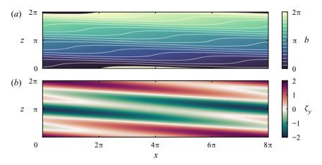
Figure 4. The initial condition of simulation U4, where s = 0.75. (*a*) Contours and colour map of the total buoyancy field  $b = z + \theta \mod 2\pi$ . (*b*) Colour map of the spanwise vorticity  $\zeta_y = \partial u/\partial z - \partial w/\partial x$ .
