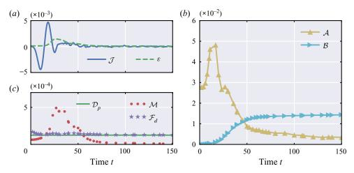
Figure 5. Energy budgets for simulation U1. (a) Time series of the mean buoyancy flux and viscous dissipation rate; (b) time series of the BPE budget terms; (c) time series of APE and BPE defined in (2.20) and (2.21). The time series for  $\mathcal{B}$  is shifted by  $-\mathcal{B}(0)$  for clarity. Terms denoted by symbols are computed from full flow output files, and so have lower time resolution than  $\mathcal{J}$  and  $\varepsilon$ , which are computed 'on the fly'.
