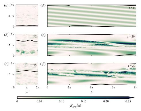
Figure 7. Vertical plane snapshots of  $E_{APE}$  as defined in (2.24). Solid lines in each case denote the isopycnal boundary  $z_1$  from which the APE is calculated. Snapshots from the forced simulations are each taken at time  $t \approx 150$  with runs F1, F2 and F3 shown in (*a*), (*b*) and (*c*) respectively. Panels (d-f) display the evolution of  $E_{APE}$  in simulation U1 from the initial condition to the peak in mixing at time t = 30.
