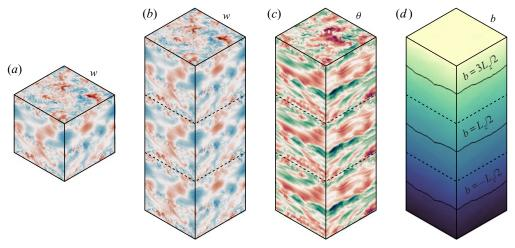
Figure 2. Example schematic of tiling the periodic computational domain vertically. The vertical velocity w, shown in (a, b), and buoyancy perturbation  $\theta$ , shown in (c), simply repeat thanks to their periodic boundary conditions. The total buoyancy  $b = z + \theta$ , shown in (d), is not periodic in the vertical, although isopycnal surfaces separated by the vertical period  $L_z$  are of identical shape.
