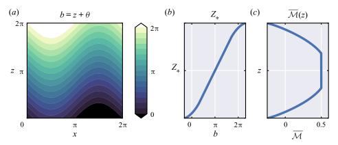
Figure 1. (a) Displays contours of the total buoyancy field given by  $\theta = \sin x$ ; (b) shows the sorted profile  $Z_*(b)$  associated with this buoyancy field; (c) shows the horizontally averaged irreversible mixing rate  $\overline{\mathcal{M}}(z) = (\overline{\partial Z_*/\partial b})|\nabla b|^2 - \partial \overline{b}/\partial z$ . Note that an overbar here denotes an average over x, and  $\partial Z_*/\partial b$  is evaluated at b(x, z).
