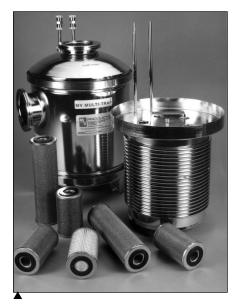
**High-Capacity Vacuum Inlet and Exhaust Trap:** The MV Multi-Trap® Model IC from MV Products is designed for collecting solids in LPCVD, MOCVD, WCVD, and metal etch processes. It provides >200 in.2 (1300 cm<sup>2</sup>) of surface area. Two customizable filtration stages condense and collect heavy particulates. The vacuum inlet and exhaust trap has >500 in.3 (8000 cm3) of space to accumulate solids. Contact: sales@massvac.com; www.massvac.com.
