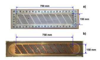
Fig. 3. Spot-welded mask on emission mesh (a) and output foil window (b).
