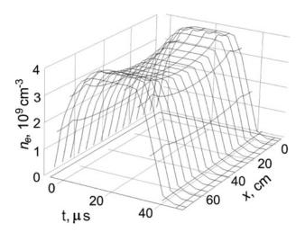
**Fig. 10.** Calculated variation of plasma density  $n_e$  with time *t* along the longitudinal axis of plasma cathode at emission mesh surface (Fig. 7, line *L*).
