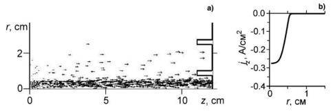
Fig. 13. The pattern of emitted and reflected electrons (a) and calculated current density distribution in one hole of output foil window (b).
