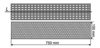
Fig. 7. Mask geometry in calculations and experiments.
