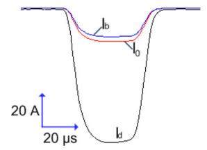
**Fig. 9.** Typical waveforms of discharge current  $I_d$ , current in accelerating gap  $I_0$ , and extracted beam current  $I_b$  at  $U_0$  = 200 kV with mask holes of diameter 8 mm, geometric transparency 13%, and h = 0.6 mm
