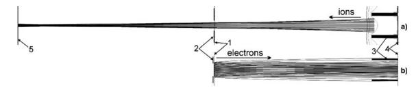
**Fig. 12.** Elementary ion (a) and electron beam configurations (b) at  $U_a = 200$  kV, h = 0.4 mm, mask and support grid hole diameters 8 mm and 15 mm, respectively: 1 – emission mesh, 2 – mask, 3 – support grid, 4 – foil, 5 – discharge hollow anode.
