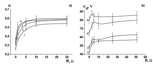
**Fig. 5.** Electron extraction factor  $\alpha$  (a) and discharge operating voltage Ud (b) versus resistance *R* in experiments with no mask at  $U_0 = 160$  kV, h = 0.4 mm, and d = 140 mm for  $I_d$  equal to 20 A (1), 40 A (2), 60 A (3), 90 A (4), 100 A (5), and 150 A (6).
