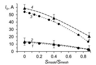
**Fig. 8.** Current in the accelerating gap  $I_0$  as a function of  $S_{mask}/S_{mesh}$  at  $U_0 = 200$  kV, h = 0.6 mm in calculations (1, 3) and experiments (2, 4) for  $I_d = 20$  A (1, 2), 90 A (3), and 100 A (4).
