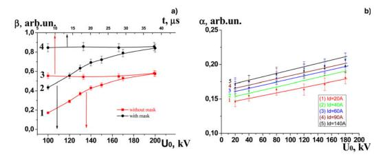
**Fig. 4.** Beam extraction efficiency  $\beta$  versus accelerating voltage  $U_0$  and beam pulse duration t at  $U_0 = 200$  kV (a) with no mask (1, 3) and with it (2, 4) and electron extraction efficiency  $\alpha$  versus  $U_0$  with mask holes of diameter 8 mm and mesh width h = 0.6 mm (b).
