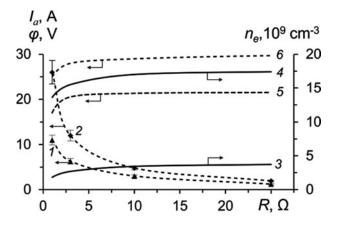
**Fig. 6.** Experimental curves for anode current  $I_a$  (1, 2) and respective calculated curves for plasma density  $n_e$  (3, 4) and plasma potential  $\varphi$  (5, 6) with respect to anode as a function of *R* at  $I_d$  = 20 A (1, 3, 5) and 100 A (2, 4, 6).
