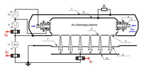
**Fig. 1.** Schematic of the electron accelerator: 1 – plasma cathode; 2 – metal cathode; 3 – igniter; 4 – emission mesh; 5 – mask; 6 – hollow anode; 7 – support grid for output foil; 8 – output foil; 9 – discharge power supply; 10 – igniter power supply; 11 – high-voltage power supply; 12 – collector or substrate.
