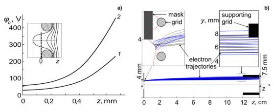
**Fig. 11.** The potential in the near-grid region due to penetration of accelerating electric field (a) at  $U_a = 100$  kV (1) and 200 kV (2), and edge effects on angular electron distribution with loose mask-to-mesh attachment (b).
