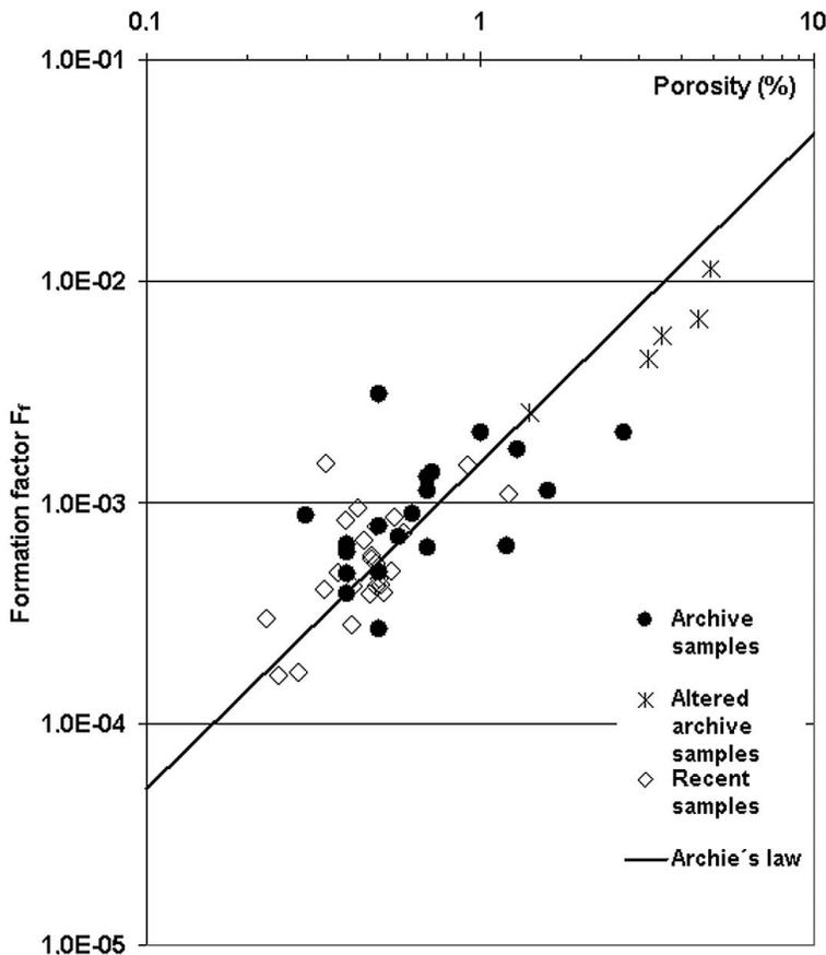
FIG. 7. Relation between the formation factor,  $F_f$  and porosity,  $\varepsilon$  in the context of sample origin. The line represents the empirical Archie's law.
