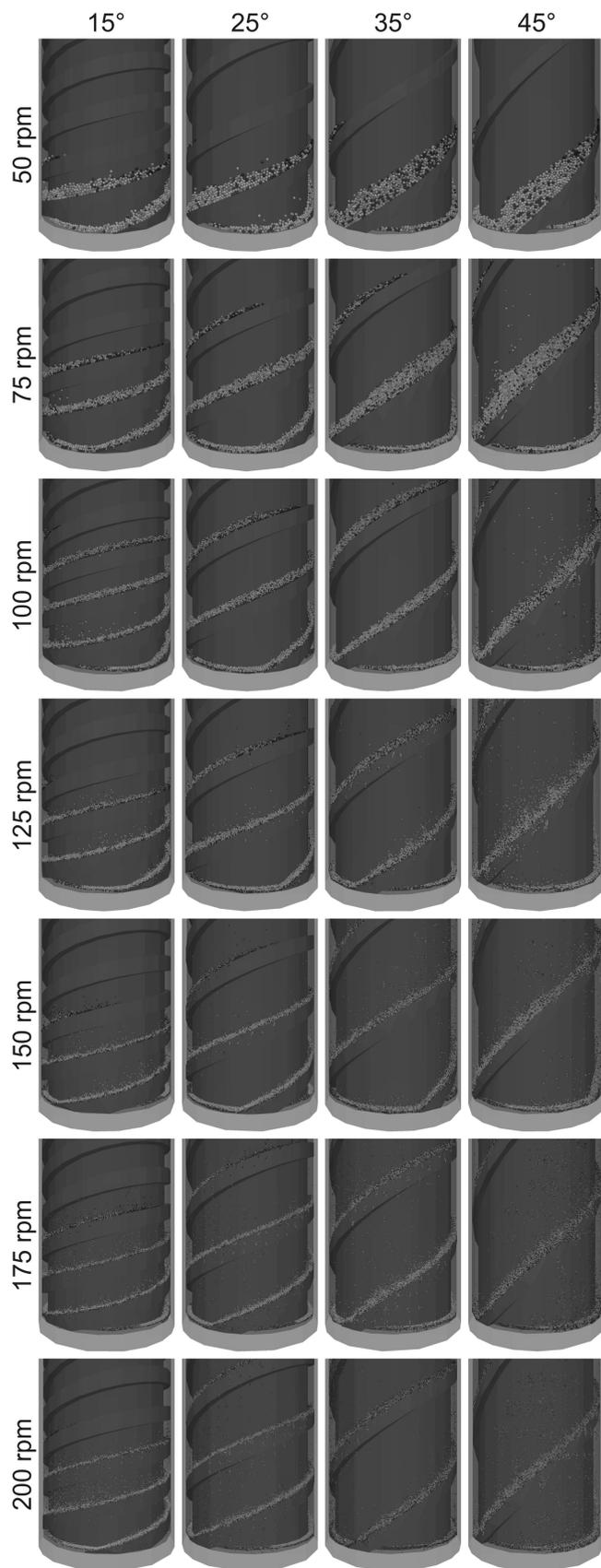
Fig. 3. Cuttings distribution along coring auger.
