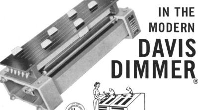
This patented Davis auto-transformer multi-dimmer coil has been the heart of Davis Dimmers for more than seven years. During that time not one has had to be returned for replacement or re-surfacing. The Davis Commutator - type coil replaces flimsy wire windings with silver-plated "C" stampings. This construction is the key'to long life and cool operation.
