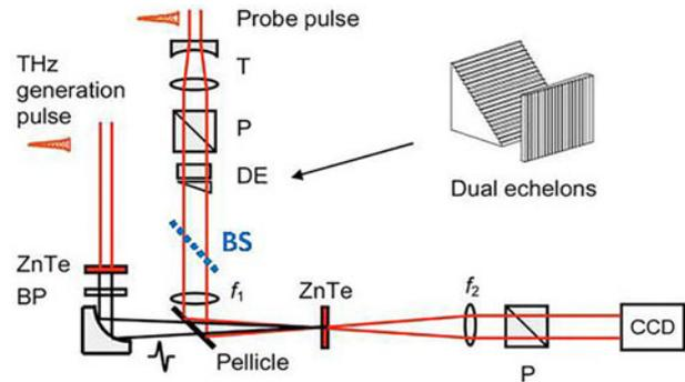
**Figure 5.** Schematic of single-shot THz measurement using dual echelon optics (quoted from Ref. [29]).
