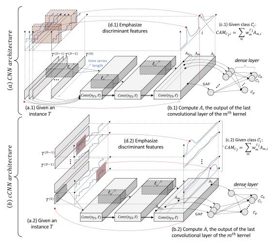
*Figure 1.* Illustration of Class Activation Map for (a) CNN architecture and (b) cCNN architecture with three convolutional layers ( $n_{f1}$ ,  $n_{f2}$ , and  $n_{f3}$  different kernels respectively of size all equal to  $\ell$ ).
