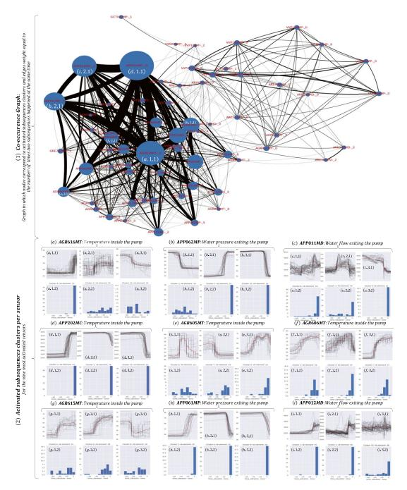
*Figure 11.* (1) Cooccurrence graph connecting the activated subsequences clusters based on their cooccurrence in time. Subsequences clusters (\*.\*.1) (and their time distribution compared to the vibration timestamps (\*.\*.2)) detected as precursors of vibration by dCAM for the nine most activated sensors.
