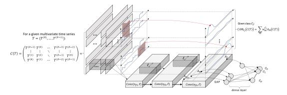
Figure 2. dCNN architecture and application of the CAM.
