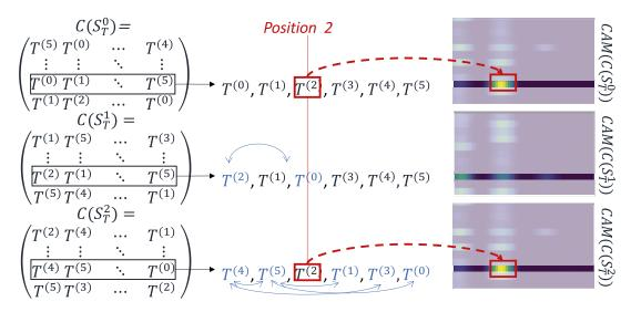
Figure 3. Example of Class Activation Map results for different permutations.
