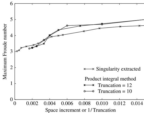
FIGURE 3. Limiting Froude number as the grid spacing is reduced (product integration method) or the truncation point is increased (singularity extraction method) (limiting  $F$  is plotted against  $1/\text{truncation point}$ ). There is no reason why the truncation curve should match the grid spacing curves except as they all approach zero on the horizontal axis.
