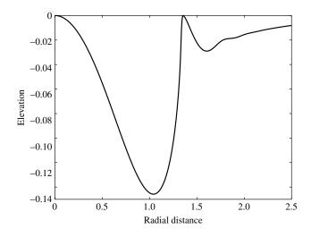
FIGURE 1. Limiting shape of the free surface F = 6.35 recomputed using the values in [3]. A uniform grid spacing of  $\Delta s = 0.04$  and a truncation point of tr = 6.0 were used to obtain this figure.
