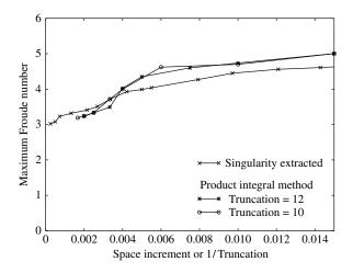
FIGURE 3. Limiting Froude number as the grid spacing is reduced (product integration method) or the truncation point is increased (singularity extraction method) (limiting F is plotted against l/truncation point). There is no reason why the truncation curve should match the grid spacing curves except as they all approach zero on the horizontal axis.
