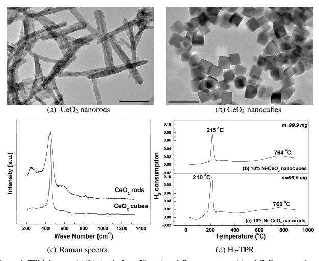
Figure 1 TEM images (a)/(b) (scale bar: 50 nm) and Raman spectra (c) of  $CeO_2$  nanorods and nanocubes, and  $H_2$ -TPR profiles (d) of 10wt% Ni/CeO<sub>2</sub> nanorods and nanocubes under a  $5\%H_2/95\%$  Ar gas atmosphere.
