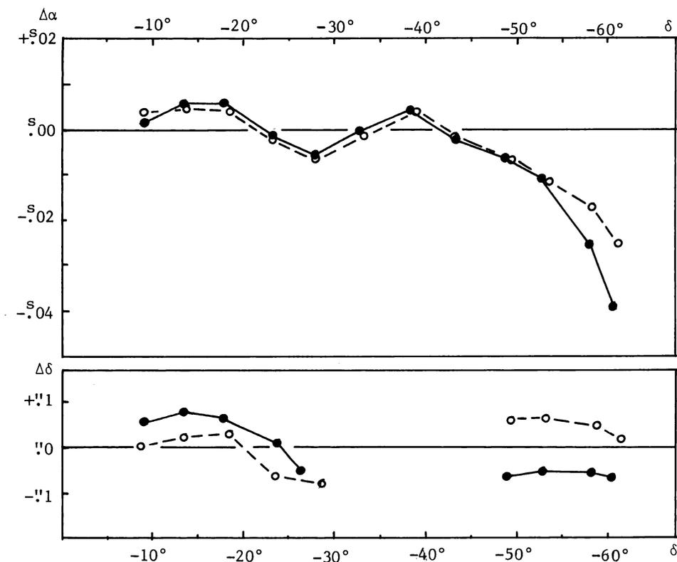
Figure 3. The  $\Delta\alpha_\delta$  and  $\Delta\delta_\delta$  errors of FK4 as obtained by the astrolabes of Santiago (—●—) and Cape (—○—) (1967.3).
