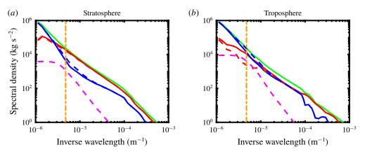
FIGURE 1. Vortical and wave energy spectra in the (a) lower stratosphere and (b) upper troposphere using the linear (solid) and nonlinear (dashed) decompositions. Spectra are wave (red), vortical (blue), total (green) and ageostrophic QG (magenta). The assumed vertical structure is the fourth baroclinic mode, and the associated deformation wavenumber is indicated with the vertical line. Adapted from Wang & Bühler (2020).
