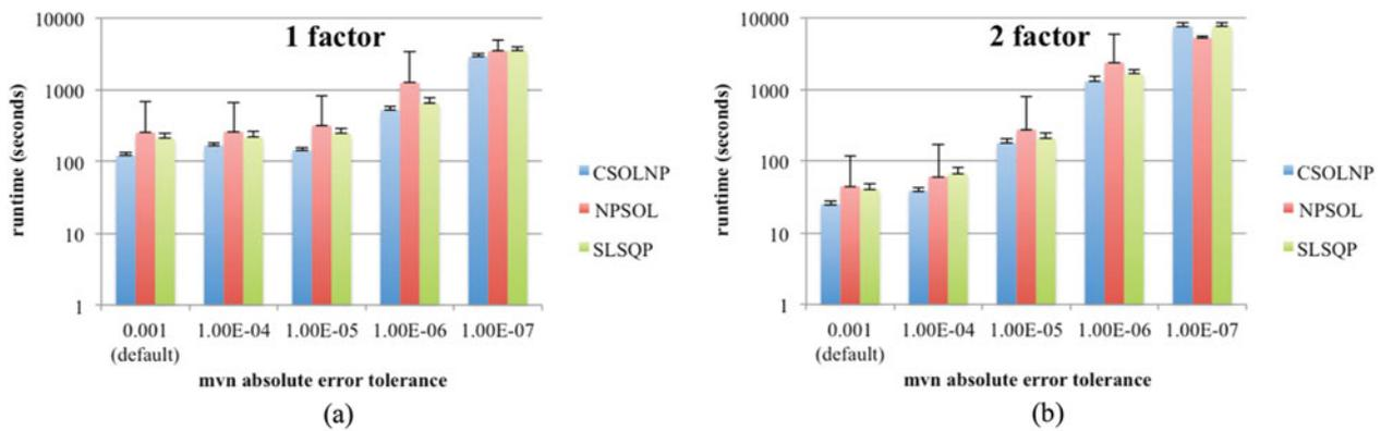
**FIGURE 3** (Colour online) Runtimes of CSOLNP, NPSOL, and SLSQP in logarithmic scale for threshold models with (a) five variables and one factor, and (b) five variables and two factors for a sample of size of 10,000. Runtimes are averaged over 250 different runs.
