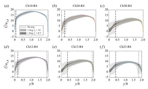
*Figure 12.* Mean velocity. The shades show the variation of the mean velocity when the data are not subjected to any spatial filtration, when the data are subjected to streamwise filtration of  $l_x = 14h$  and when the data are subjected to spanwise filtration of  $l_z = 8.5h$ .
