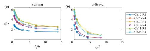
*Figure 13.* The error in the mean velocity when one applies (a) streamwise averaging of size  $l_x$  and (b) spanwise averaging of size  $l_z$ .
