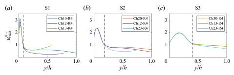
**Figure 11.** Dispersive stress  $u''_{rms}$  near S1, S2 and S3. The plots cutoff at y/h = 1 or  $\langle U \rangle = \max[\langle U \rangle]$ . Here, normalization is by the friction velocity  $u_{\tau}$ .
