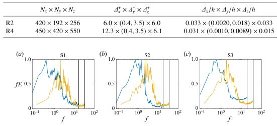
**Figure 5.** Premultiplied roughness spectra. The spectra are normalized by their maxima. The blue lines are the x direction spectra. The yellow lines are the z direction spectra. The vertical lines denote the grid cutoff in the  $Re_{\tau} = 395$  DNSs.
