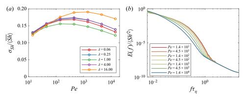
Figure 3. Second-order statistics of transfer rate fluctuations Sh'. (a) The standard deviation of transfer rate fluctuations with respect to the mean, as a function of Péclet number. (b) The power spectral density of the transfer rate fluctuations for spherical particles at varying Pe.
