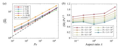
Figure 2. Mass transfer coefficient for small spheroids in a turbulent flow. (a) The scaling of ensemble-average Sherwood number with turbulent Péclet number for five different aspect ratios  $\lambda$ , compared to the expected  $\langle Sh \rangle \sim Pe^{1/3}$  scaling for steady flows. (b) The dependence of the ensemble-average mass transfer rate  $\langle \overline{Sh} \rangle$  upon the aspect ratio  $\lambda$ , compensating for the expected  $Pe^{1/3}$  scaling.
