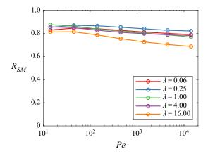
Figure 8. Correlation coefficient between transfer rate obtained from quasi-steady flux model and numerical simulation.
