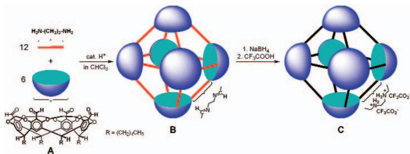
Figure 1. An octahedral nanocontainer (**B**) composed of six cavitands (**A**) linked together with 12 diamino bridges via 24 newly formed imine bonds; **B** is reduced to polyamino nanocontainer (**C**).
