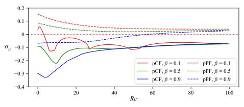
Figure 5. Influence of weak inertia on linear instability of pCF and pPF at Wi = 2.5 and Wi = 4.0, respectively, at  $k_1 = 0.65$  as denoted by the green cross in figure 3. The dotted red line denotes marginal stability.
