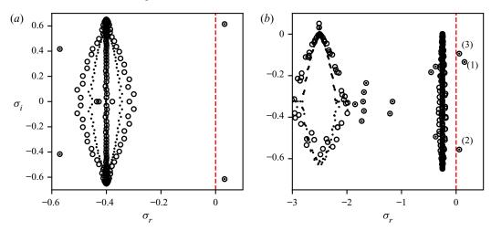
Figure 1. Eigenvalue spectra for  $\beta = 0.1$  and  $k_1 = 0.65$  for (a) pCF at Wi = 2.5, and (b) pPF at Wi = 4.0. The dashed red lines denote marginal stability. Both figures compare spectra calculated with 50 (open circles) and 100 (dots) Chebyshev polynomials.
