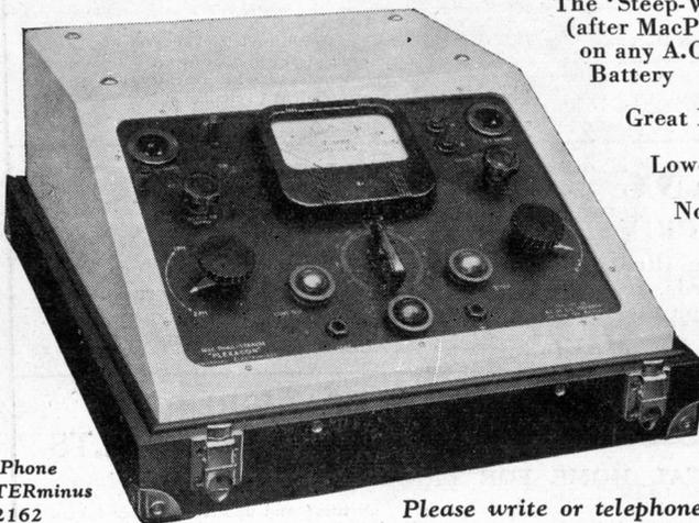
The 'Steep-Wave' Electroplexy Unit (after MacPhail & Strauss) operates on any A.C. or D.C. Supply or 12v. Battery
