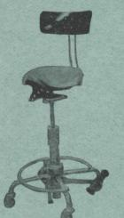
Hydraulic, Foot Operated Adjustable Height 24 to 33 inch Adjustable Back Rest Foot Operated Brake Foot Rail Maximum Manœuvrability Can be elevated and locked by Surgeon whilst seated
