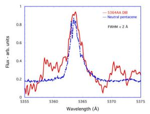
**Figure 4.** Comparison of band profiles of jet-cooled pentacene ( $C_{22}H_{14}$ ) with CRDS and the 5363.8 Å DIB measured with the OHP echelle spectrograph (see text). The laboratory band (dotted line) was slightly shifted in wavelength for illustration purposes. Taken from Salama (2008).
