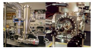
**Figure 2.** Configuration of the Laboratory Facility. *Right:* close-up view of the Chamber consisting of a Pulsed Discharge Nozzle coupled to a Cavity Ringdown Spectrometer apparatus and Reflectron time-of-flight mass spectrometer.
