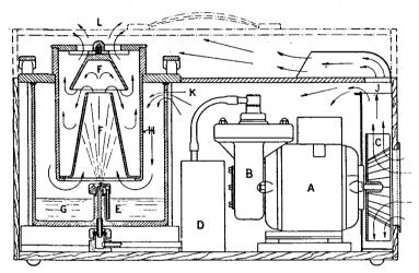
Fig. 1. Vertical section of Dynalysor.
