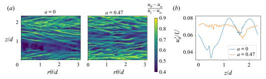
FIGURE 8. (a) Instantaneous normalized azimuthal velocity at  $r^+=15$  for  $Ta=5\times 10^8$  for a=0 ( $R_\Omega=0.09$ ) and a=0.47 ( $R_\Omega=0.03$ ). The DNS corresponds to the case of  $\Gamma=2.33$ . (b) Azimuthal average of the root-mean-squared azimuthal velocity  $u_\theta'$  as a function of axial position at  $r^+=15$  for the two values of rotation a. A clear break in axial homogeneity can be appreciated for a=0.
