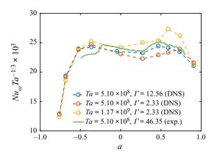
FIGURE 9. Compensated Nusselt number as a function of a obtained from the DNS of the current study. The green solid line is the experimental data performed at  $Ta = 5.10 \times 10^8$ .
