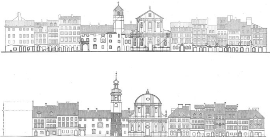
Figure 4. Elevation of Piwna Street in Warsaw based on surveys conducted in 1939 and after 1944 (top), juxtaposed with as-built drawings from 1956 (bottom). After Biegański and Zachwatowicz (eds.), Stare Miasto w Warszawie , personal collection of J. Elżanowski.
