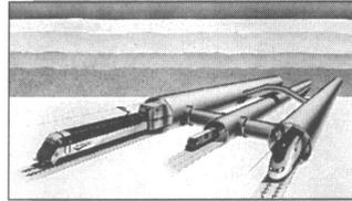
Schematic drawing of the Channel Tunnel (By permission of Eurotunnel)
