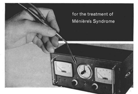
PROBE - 2mm. diameter beam produced by micro-cone concentrator gives precisely controlled energy pattern ■ Incorporates saline irrigation tube Built-in thermistor thermometer monitors saline temperature E Finished in stainless steel and sealed for autoclave sterilisation
