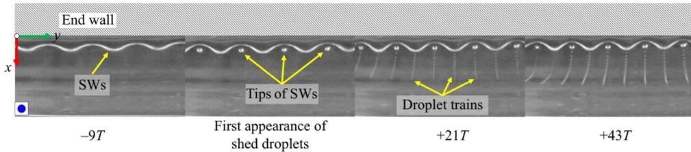
Figure 7. Sequence of top-view images showing how droplets are shed from the crests of SWs in the fluid pair HT135-SO100 for  $f = 25$  Hz ( $T = 0.04$  s) and  $A = 1.07A_c = 2.65$  mm. The snapshots are taken when the container at its leftmost position (blue circle as in figure 3) and the first image is captured while the SWs are still developing.
