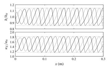
FIGURE 7. Spatial development of the film height  $h/h_N$  and the streamwise velocity at the interface  $u_{\Sigma}/u_N$  for case A2 (Re = 5.2), obtained with DNS. The minimum and maximum values at the measurement position ( $x_m = 0.256$  m) are shown as a reference by the dashed grey lines.
