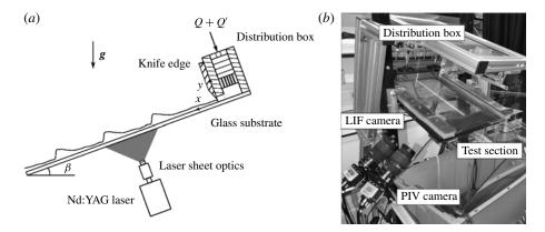
FIGURE 2. (a) Schematic of the test section and part of the flow loop. (b) Test section arrangement showing the position of the cameras and illuminated region of the film (Charogiannis *et al.* 2015, 2017).
