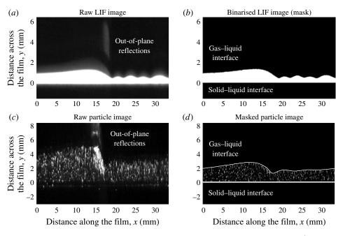
FIGURE 3. (a) PLIF image from a flow with Re = 62, Ka = 350 and  $f = 10 \text{ s}^{-1}$ , following corrections for refractive-index and perspective distortions, and (b) binarised PLIF image after removal of out-of-plane reflections. (c) Particle image from a flow with Re = 24, Ka = 85 and  $f = 10 \text{ s}^{-1}$  after corrections for refractive-index and perspective distortions, and (d) masked-particle image using its processed PLIF counterpart.
