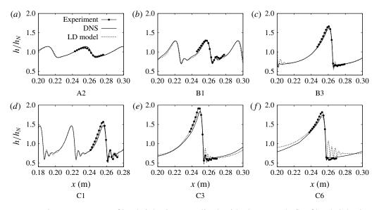
FIGURE 9. Instantaneous film height h, normalised with the Nusselt flat-film height  $h_N$ , for selected cases as a function of downstream distance x.
