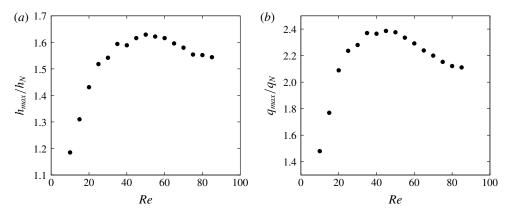
FIGURE 13. Maximum film height  $h_{max}$  (a) and maximum flow rate  $q_{max}$  (b), normalised by the corresponding Nusselt solution, as a function of Reynolds number *Re* for case C with  $f = 10 \text{ s}^{-1}$ , obtained with DNS.
