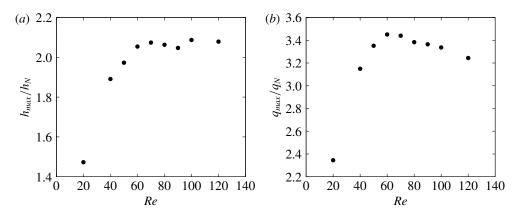
FIGURE 14. Maximum film height  $h_{max}$  (a) and maximum flow rate  $q_{max}$  (b), normalised by the corresponding Nusselt solution, as a function of Reynolds number *Re* for a falling water film on a vertical substrate, as previously considered in Denner *et al.* (2016), obtained with DNS.
