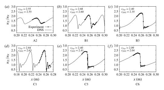
FIGURE 10. Instantaneous streamwise interface velocity  $u_{\Sigma}$ , normalised with the Nusselt velocity  $u_N$ , for selected cases as a function of downstream distance x. The wave speeds measured in the experiments,  $c_{Exp}$ , and the DNS,  $c_{DNS}$ , are given as well.
