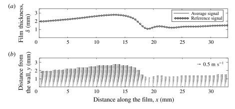
FIGURE 4. (a) Reference and average-wave profiles for a film with Re = 26.9, Ka = 85 and a 10 s<sup>-1</sup> forcing frequency. (b) Average PTV-derived velocity field corresponding to the average film-thickness profile in (a).
