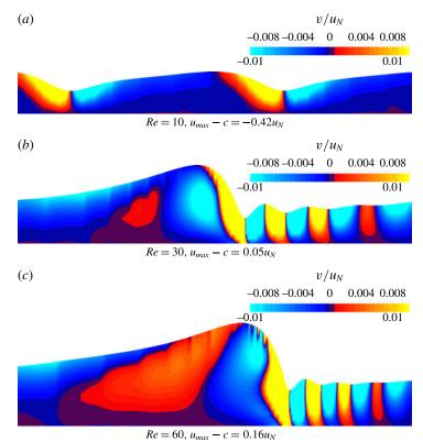
FIGURE 16. (Colour online) Cross-stream velocity v, normalised by the Nusselt velocity  $u_N$ , of case C with  $f = 10 \text{ s}^{-1}$  for  $Re \in \{10, 30, 60\}$ , obtained with DNS. No flow recirculation in the moving frame of reference is observed for Re = 10 ( $c > u_{max}$ ), but flow recirculation is present for Re = 30 and Re = 60 ( $c < u_{max}$ ). Note that the limits of the colour scale ( $-0.01 \ge v/u_N \ge 0.01$ ) do not represent the min/max values of the
