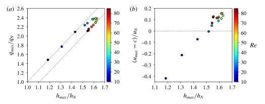
FIGURE 15. (Colour online) Maximum flow rate  $q_{max}$  (a) and relative velocity  $u_{max} - c$  (b), normalised by the corresponding Nusselt solution, as a function of maximum film height  $h_{max}$  for case C with  $f = 10 \text{ s}^{-1}$  in the range Re = 10-85, obtained with DNS. The colour scale represents the Reynolds number.
