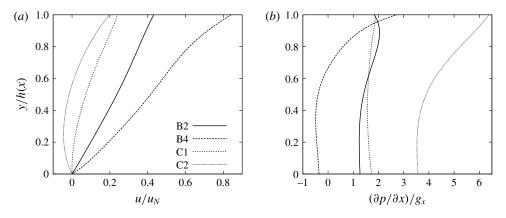
FIGURE 17. DNS profiles of the streamwise velocity  $u/u_N$  (*a*) and the streamwise pressure gradient (*b*), normalised with the streamwise component of gravity  $g_x$ , at the trough preceding the solitary wave, position X4, for cases B2 (Re = 11.7,  $f = 7 \text{ s}^{-1}$ ), B4 (Re = 26.9,  $f = 10 \text{ s}^{-1}$ ), C1 (Re = 12.4,  $f = 7 \text{ s}^{-1}$ ) and C2 (Re = 28.5,  $f = 10 \text{ s}^{-1}$ ), obtained with DNS.
