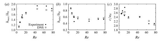
FIGURE 11. Maximum film height  $h_{max}/h_N$  (a), minimum film height  $h_{min}/h_N$  (b) and wave speed  $c/u_N$  (c) as a function of *Re* for cases with  $f = 7 \text{ s}^{-1}$ . Results obtained with the LD model are omitted in the interest of clarity.
