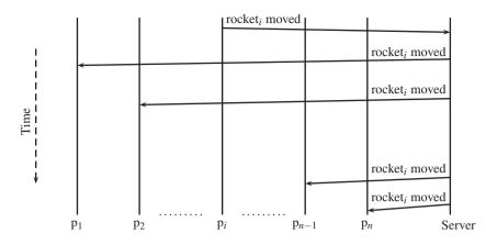
Fig. 3. Communication protocol diagram for a rocket move.
