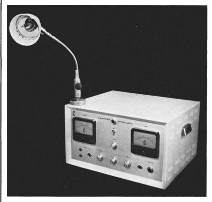
The Ahrend Van Gogh Laryngostroboscope ( $\triangle$  F Generator) shows the vibration of the vocal chords slowed down to about one cycle per second. It is also possible to stop the movement by stroboscopic effect and then tune through all phases of one cycle.
