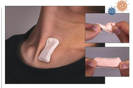
Soft, wireless electronic sensor mounted on the suprasternal notch enables continuous recordings of mechano-acoustic signatures of key symptoms of COVID-19—heart rate variability, respiration rate and respiratory sounds, cough (frequency, intensity), and temperature. Credit: John Rogers.
