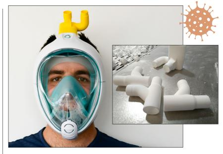
These 3D printed valves are produced by 3D Systems On Demand to convert a Decathlon snorkeling mask to an emergency ventilator mask. Designed by the company Issinova, located in northern Italy, the 3D printing instructions for the valve are available free. Full mask photo credit: Issinova. Inset credit: 3D Systems.
