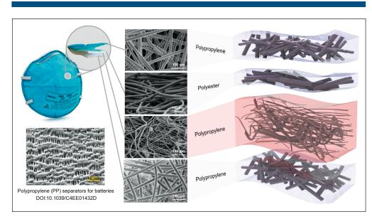
A 3M N95 mask model in comparison with a battery separator using a similar material. As polypropylene is utilized in both battery separators and masks, Shirley Meng and her research group at the University of California, San Diego, apply their tools for battery study on N95 masks as well. Credit: Shirley Meng, Min-cheol Kim, and Diyi Cheng.
