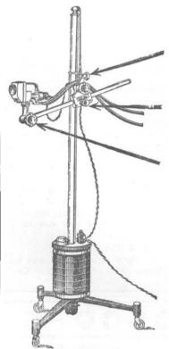
Tubular member, for raising or lowering the lamp, attached to an internal counter weight, permitting the lamp to be raised or lowered to any height desired.
