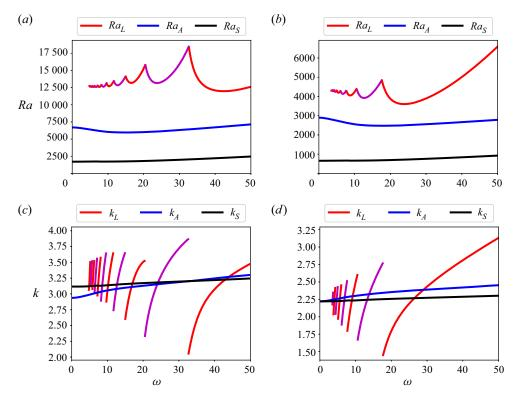
Figure 5. Temperature modulation results with Pr = 1: (a,c) no-slip; (b,d) no-stress. For  $Ra_L$ , magenta indicates a synchronous disturbance (i.e.  $Im(\mu) = 0$ ) and red indicates a subharmonic disturbance (i.e.  $Im(\mu) = 1/2$ ).
