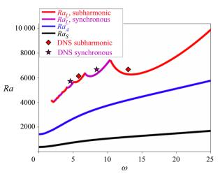
Figure 10. Validation of the competition between synchronous and subharmonic modes. The analytical results come from figure 2(b). Symbols show corresponding unstable numerical simulations performed for a Rayleigh number just above the threshold. A complete list of DNS parameters is provided in table 1.
