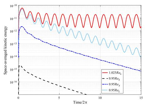
Figure 9. Temporal evolution of the space-averaged kinetic energy as a function of time for four DNS runs illustrating the linear and nonlinear stability regimes at  $\omega = 100$ , Pr = 1.0, and for Ra = 1.025  $Ra_L$ , 0.95  $Ra_A$  and 0.95  $Ra_A$  and 0.95  $Ra_S$ , respectively. Values of  $Ra_L$ ,  $Ra_A$  and  $Ra_S$  come from the analytical study (figure 3). A complete list of parameters is provided in table 1.
