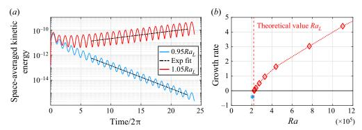
Figure 8. Linear stability study for  $\omega = 100$  and Pr = 1.0. (a) Two examples of the time evolution of the space-averaged kinetic energy and of the determination of the exponential growth rate. (b) Measured growth rate as a function of the Rayleigh number for 9 runs. A complete list of parameters is provided in table 1.
