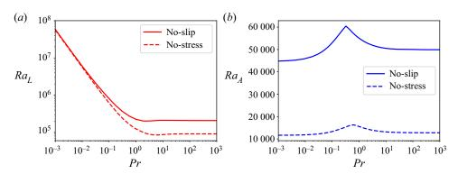
Figure 4. Dependence of (a)  $Ra_L$  and (b)  $Ra_A$  on Pr for  $\omega = 100$ , with symmetric no-slip and no-stress conditions, and heat-flux modulation.
