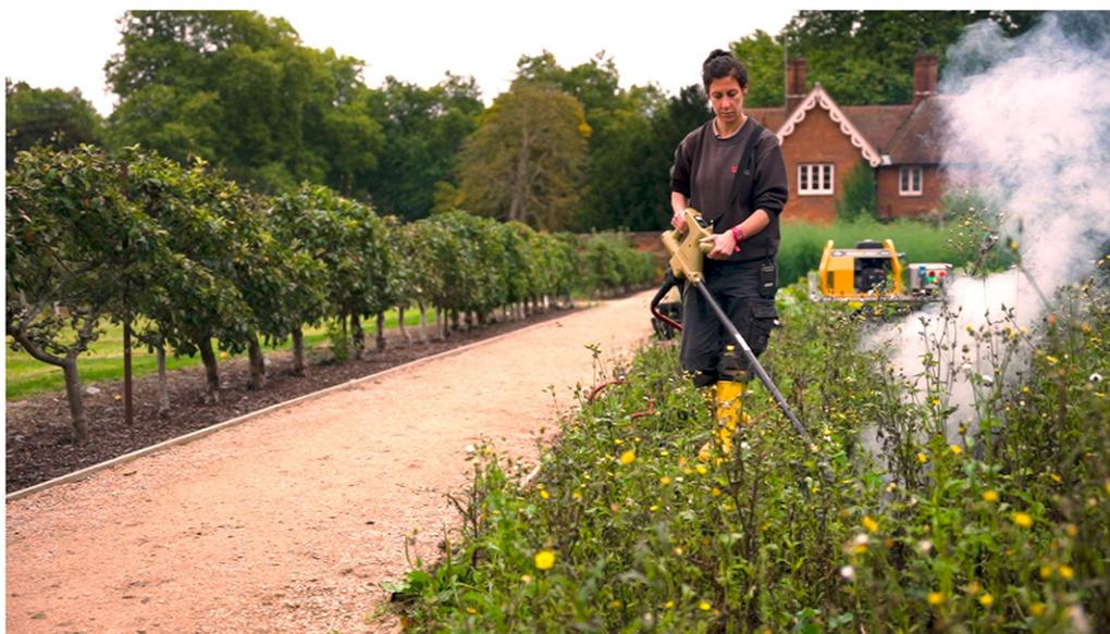
**Figure 11.** The RootWave™ handheld electric weeder, the RootWave™ Pro (Table 1). Image sourced from T. Archer (personal communication, April 2, 2022).
