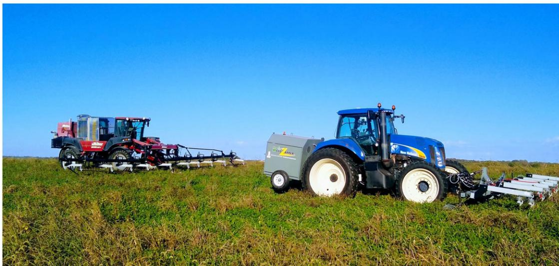
**Figure 6.** The Weed Zapper™ electric weed control machine, produced by Old School Manufacturing (Table 1). The image includes the Annihilator Tractor Series (right, 12R30 model) and the Terminator Self-Propelled Series (left, T3 model), each fitted with flexible front applicator booms of 9.1 and 18.3 m (30 and 60 feet), respectively. The image is sourced from B. Kroeger and N. Kroeger (personal communication, March 25, 2022).
