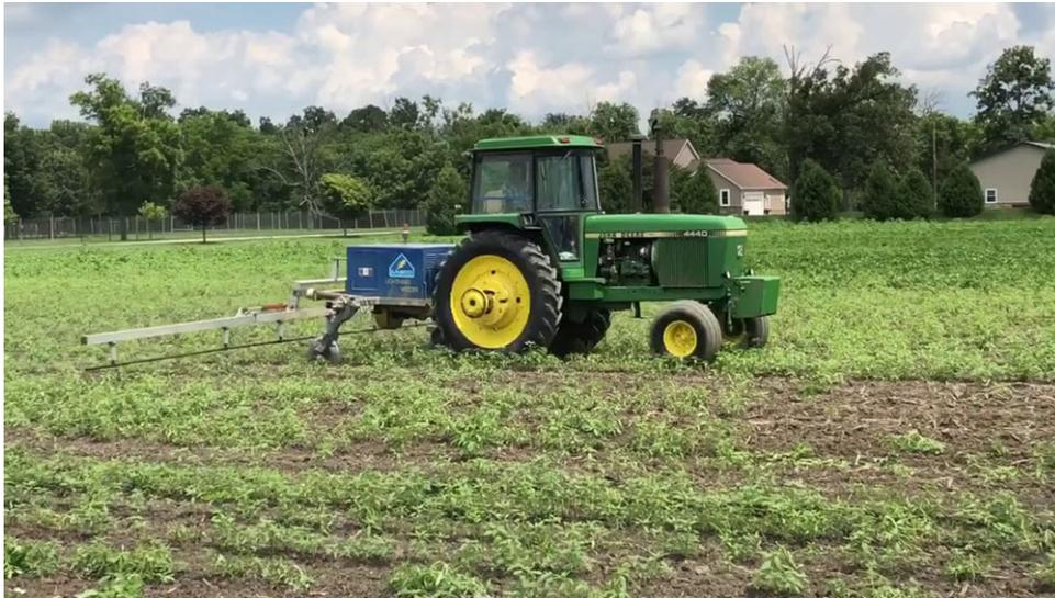
**Figure 5.** The electric weed control machine, the Lightning Weeder, developed by Lasco (Table 1). Image sourced from Lasco (2021).
