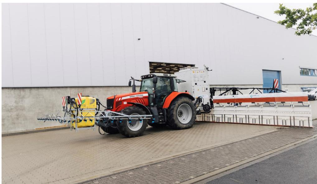
**Figure 7.** crop.zone and Nufarm's electrochemical weeding machine, NUCROP (Table 1). Image sourced from D. Vandenhirtz (personal communication, September 10, 2021).
