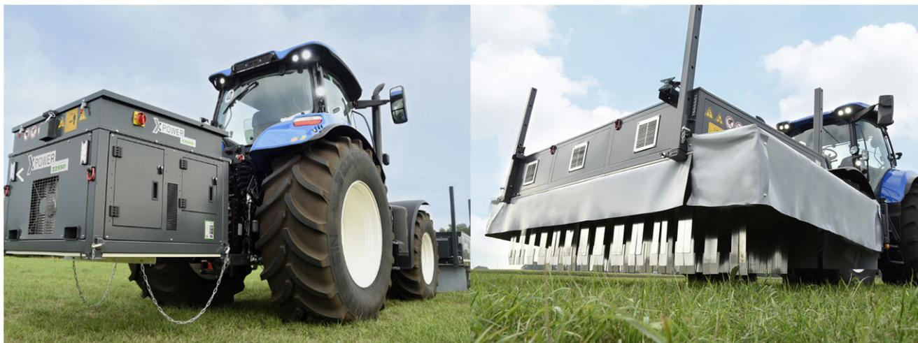
**Figure 10.** The XPower electric weed control machine with the XP300 applicator, developed by Zasso™ (Table 1). Images sourced from Zasso Group AG (2021a).
