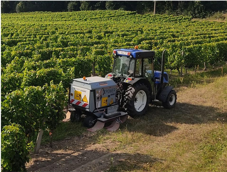
**Figure 8.** The XPower electric weed control machine with an XPS applicator, developed by Zasso™ (Table 1). Image sourced from Zasso Group AG (2021i).
