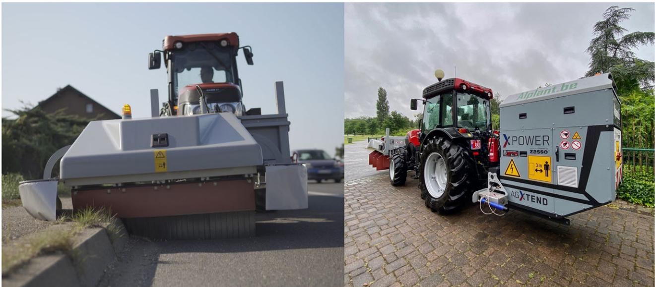
**Figure 9.** The XPower electric weed control machine with the XPU applicator, developed by Zasso™ (Table 1). Images sourced from Zasso Group AG (2021g).
