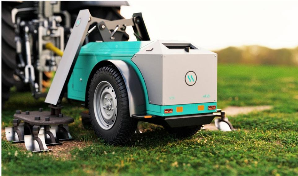
**Figure 12.** The RootWave™ vineyard and orchard electric weeder, the RootWave™ Top Fruit (Table 1). Image sourced from RootWave™ (2023a).
