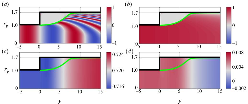
FIGURE 2. (a,b) Real part of the entropy perturbation for: (a)  $S_t = \omega R_u / \bar{u}_0 = 0.5$  and (b)  $0.0125$  – results are from the bespoke simulation. (c) Mean pressure from RANS simulation and (d) real part of the perturbation pressure at  $S_t = 0.0125$  obtained by full LNSE simulations. The green line denotes the separation streamline.
