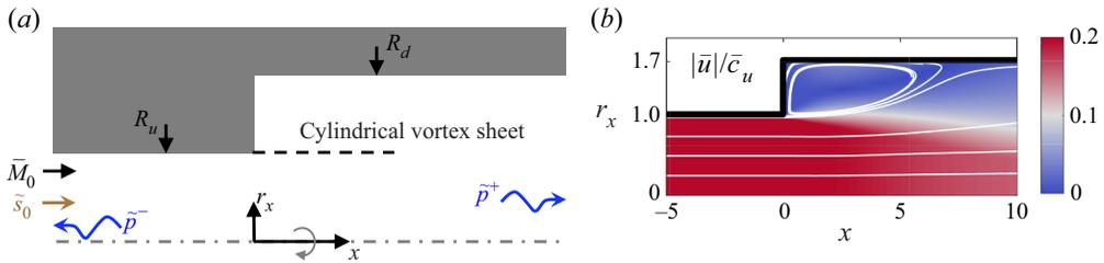
FIGURE 1. (a) A schematic view of an axisymmetric flow expansion with an incoming mean flow  $\bar{M}_0$  and entropy wave  $\tilde{s}_0$  imposed at the inlet, and generated acoustic waves  $\tilde{p}^\pm$ . (b) Magnitude of the normalised mean velocity field. The white lines denote streamlines.
