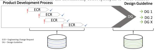
Figure 1: Product development process displaying the database capture of ECRs and DGs.
