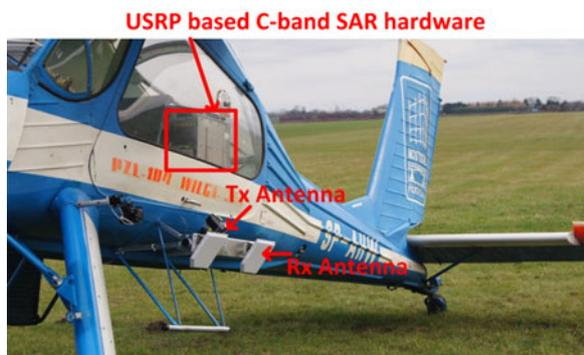
Fig. 13. The radar installation on PZL-104 Wilga aircraft.
