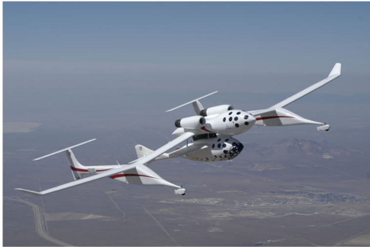
Figure 6. The White Knight turbojet aircraft with SpaceShipOne attached below (Courtesy of Scaled Composites, LLC).
