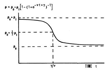
Fig. 4. Correlation,  $\rho$ , as a logistic function of time:  $\rho_0$  and  $\rho_1$  are interpreted as components of correlation, and  $\nu$  and  $\gamma$  control the rate and timing of attenuation of  $\rho_1$ .
