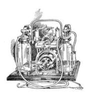
The outstanding feature of this apparatus is that there are two separate pairs of cylinders for pressure and for suction, without intercommunication between them; so the pressure cylinders cannot possibly become contaminated by anything that has been drawn away from any patient.
