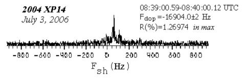
Figure 6. The measurement of Doppler shift of NEA 2004 XP14 echo received with Evpatoria RT-70. The echo-signal is cross-correlated with model of sounding signal of Goldstone RT-70; correlation coefficient R (y axes) is plotted vs. Doppler shift Fsh (x axes).
