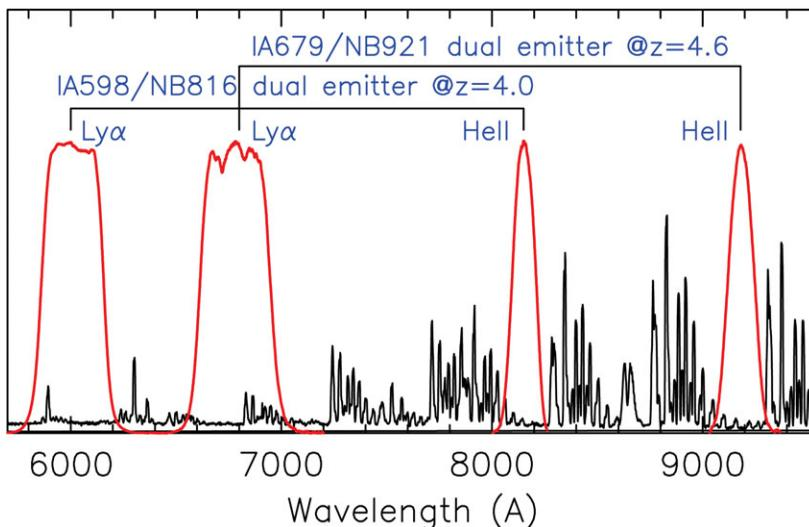
**Figure 1.** Schematic view of our selection method for Ly $\alpha$ -HeII dual emitters. The black solid spectrum denotes a typical sky spectrum. Red solid curves denote the filter transmission curves of IA598, IA679, NB816, and NB921. The dual excess of the combination of IA598 and NB816, and that of IA679 and NB921 corresponds to  $z \sim 4.0$  and  $z \sim 4.6$ , respectively.
