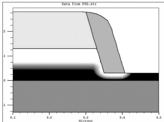
Figure 2. Ultrashallow source/drain extensions (a) micrograph and (b) schematic.
