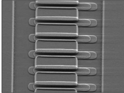
Figure 1. Scanning electron micrograph showing an interdigitated Flexfet device with self-aligned TiN top and silicon bottom gates in trenches between source/drain mesas; image made prior to local interconnect and metallization.
