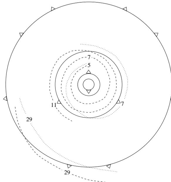
Fig. 5. Fragments early in the spirals of primes resulting from the two alternative wheel-changing rules: the dotted spiral traces Mark I, and the dashed spiral Mark II. ( $W_3$  is shown *half-size* to resolve a conflict of scale.)
