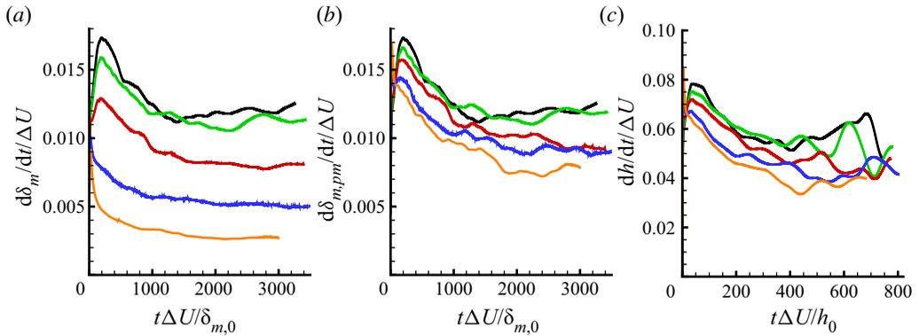
FIGURE 4. Time evolution of mixing layer thickness growth rates based on (a) momentum thickness  $\delta_m$ , (b) momentum thickness per unit mass  $\delta_{m,pm}$  and (c) mean velocity thickness  $h$ . These correspond to the time derivatives of the thickness evolutions shown in [figure 3](#).
