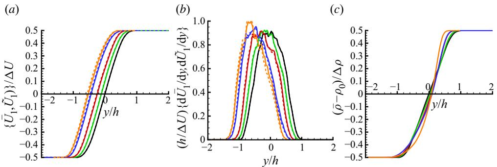
FIGURE 9. Self-similar time-averaged profiles for all Atwood numbers showing (a) mean streamwise velocity, (b) its  $y$  gradient and (c) scaled mean density. In (a) and (b), the solid line represents Reynolds mean, while the dashed line represents Favre mean. Lines are coloured by Atwood number as in figure 3.
