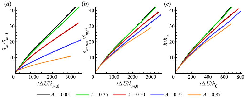
FIGURE 3. Mixing layer widths: (a) momentum thickness  $\delta_m$ , (b) momentum thickness per unit mass  $\delta_{m,pm}$  and (c) mean velocity thickness  $h$  time evolution for each Atwood number. Lines are coloured by Atwood number:  $A = 0.001$  (black);  $A = 0.25$  (green);  $A = 0.50$  (red);  $A = 0.75$  (blue);  $A = 0.87$  (orange).
