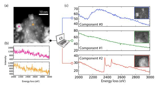
**Figure 1.** (a) TEM-EELS analysis of a fuel cell cathode material containing nano-particulate platinum and niobium oxide on a  $NbO_x$ -carbon hybrid support. (b) The raw spectral data are noisy due to limited beam dose to avoid sample damage. (c) ICA finds three main components in the spectral mixture, belonging to platinum and niobium.
