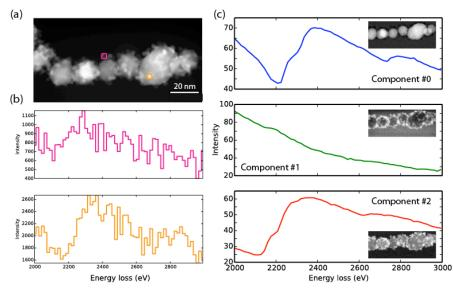
**Figure 2.** (a) TEM-EELS analysis of a AuPt nanoparticle ensemble. (b) Trace evidence of gold and platinum edges are present in the noisy raw EELS spectra. (c) ICA successfully separates the spectrally and spatially overlapping gold and platinum edges in the EELS signals present in the raw data.
